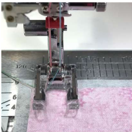
1. Manually Thread both needles, one at a time. Place stabiliser behind fabric
