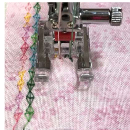
3. Select another decorative stitch, notice that you cannot choose 'greyed out' patterns. Sew across the block
