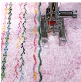
4. Repeat for other stitch patterns, lining up the edge of the foot with the previous stitches
