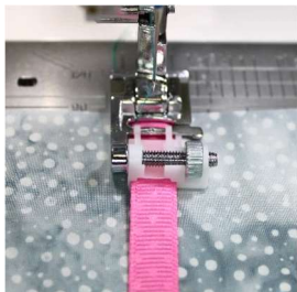
1. Insert the ribbon into the lowest section of the foot. Position the foot in the middle of the block.
