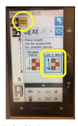
**Note:** Machines without AcuFeed and Sewing Applications, use your ¾" seam foot and select a piecing stitch, length 1.8mm. Stitch width, set your stitch line to 6mm from the fabric edge when piecing. Set your foot pressure as per your machine instruction
