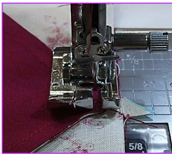
No guide O foot: smoothly sew the overlapping seam allowance parts.
