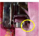
Raise the foot, using the Foot up/down button and insert the folded portion of the fabric into the slit of the foot. Lower the foot while pulling the folded portion of the fabric slightly to the left.
