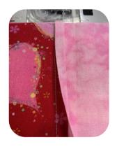
Fold the seam allowance to the left, place under the foot, sew several stitches slowly, aligning the seam line with the guideline on the foot, then stop with the needle in the down position.
