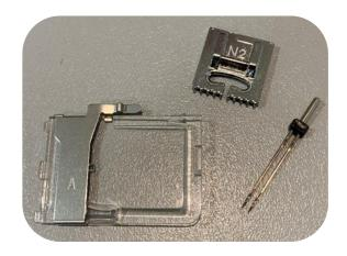
Remove the Bobbin cover plate from the machine. Insert bobbin wound with thread for pintucking. Attach the **Pintucking Cord Guide 'A'**Change the needle to the <u>Twin needle 2mm</u>
