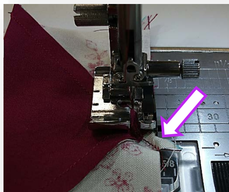
Normal O foot: Seam allowance can get caught in guide plate.
